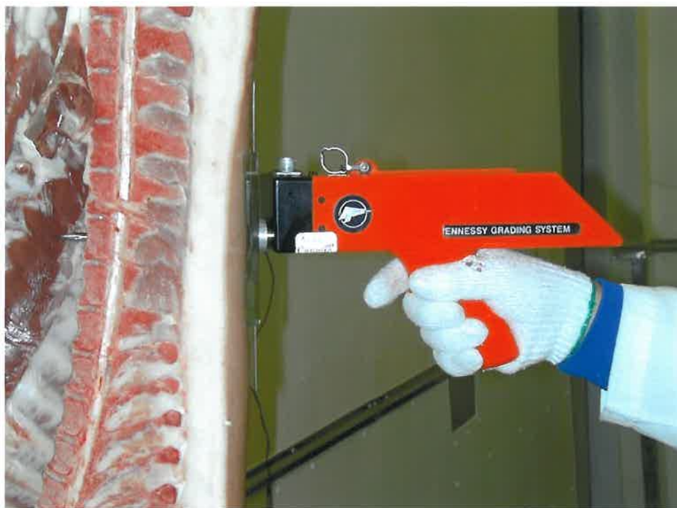
Figure 1. Measuring thickness of backfat and muscle at the 3 rd /4 th last rib using the Hennessy Grading Probe.
