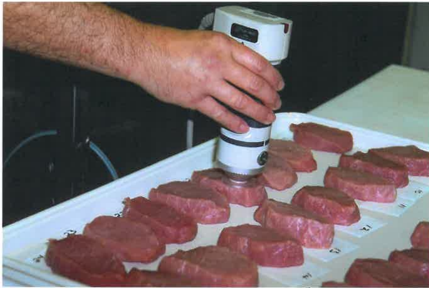
Figure 5. Measuring meat color using the Minolta CR-300 reflectance meter
