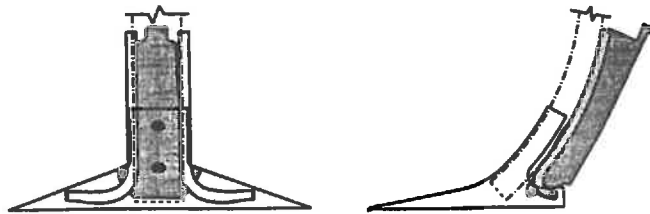
Anhydrous Ammonia tubes set-up
