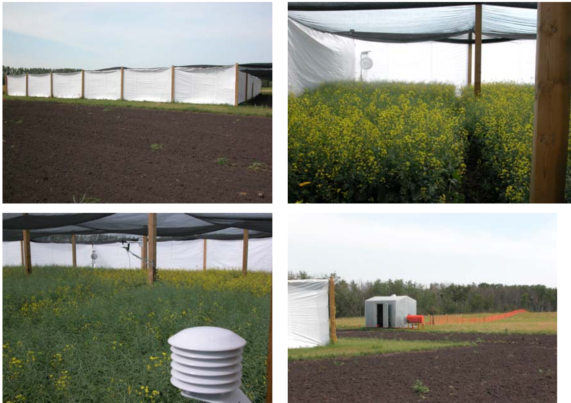
Figure 3 Modifications to the nursery design in 2007. Upper left photo shows the solid walls that replaced the permeable shade cloth side walls used in 2006. Photos on the upper right and lower left are interior view of the nursery showing the solid walls and the additional misting unit installed in 2007; Campbell Scientific instrumentation is also visible in the latter image. The diesel generator used to power the nursery is seen in the lower right image; water tanks were not necessary in 2007 as the nursery was supplied directly from municipal water supply.
