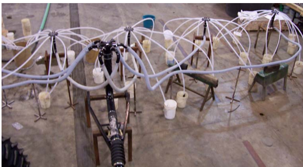
Figure 5. Air Kit Mounted on Test Stands.
