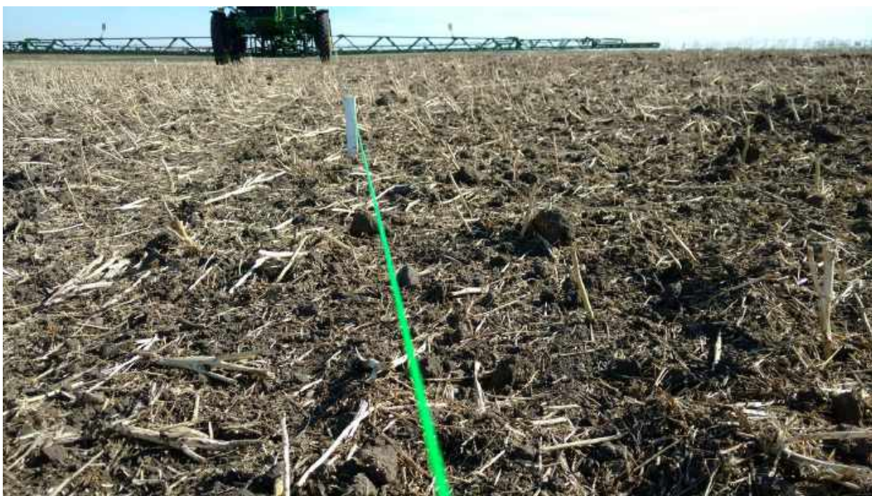
Figure 73: String collector placement adjacent to sprayer wheel
