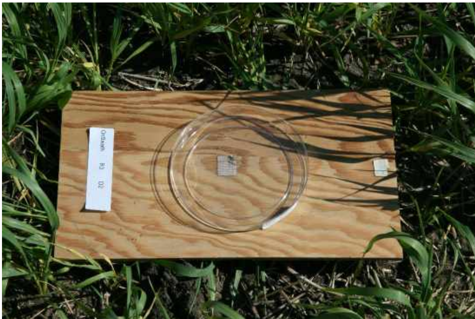
Figure 63: On swath deposit collected on 15 cm petri plates
