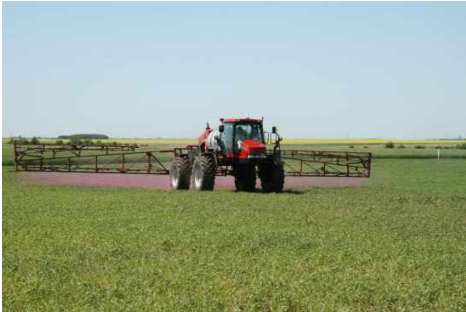
Figure 62: Spray drift tests included measurement of on swath deposit variability
