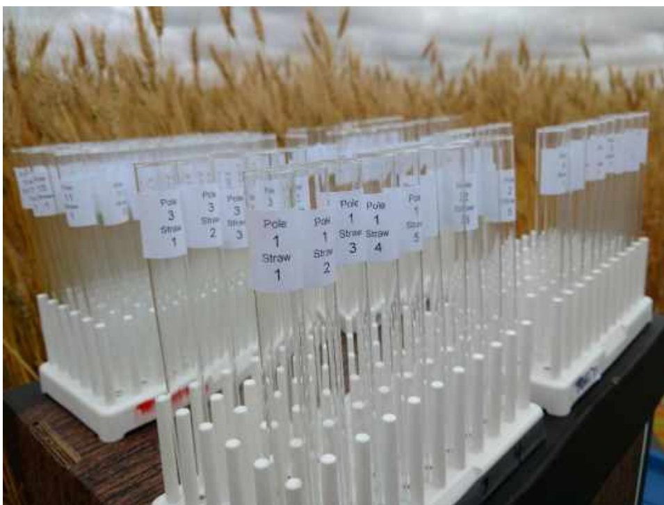
Figure 70: Borosilicate tubes to hold exposed samplers and extract dye using solvent
