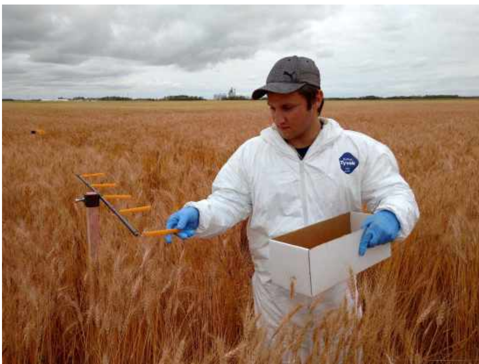
Figure 69: Placement of plastic drinking straw samplers onto sampling pole
