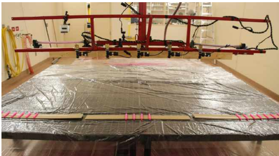
Figure 64: AAF Track Room for dynamic spray pattern testing.
