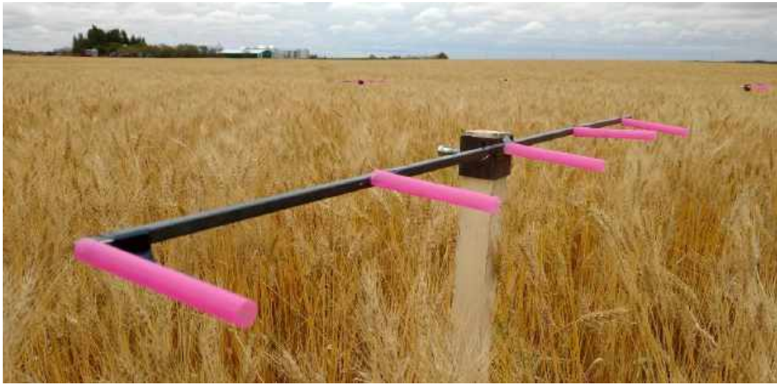
Figure 6: One m wide sampling pole with samplers spaced 25 cm apart
