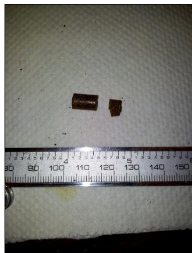
Fig. 2.2: Pellet after drop testing
