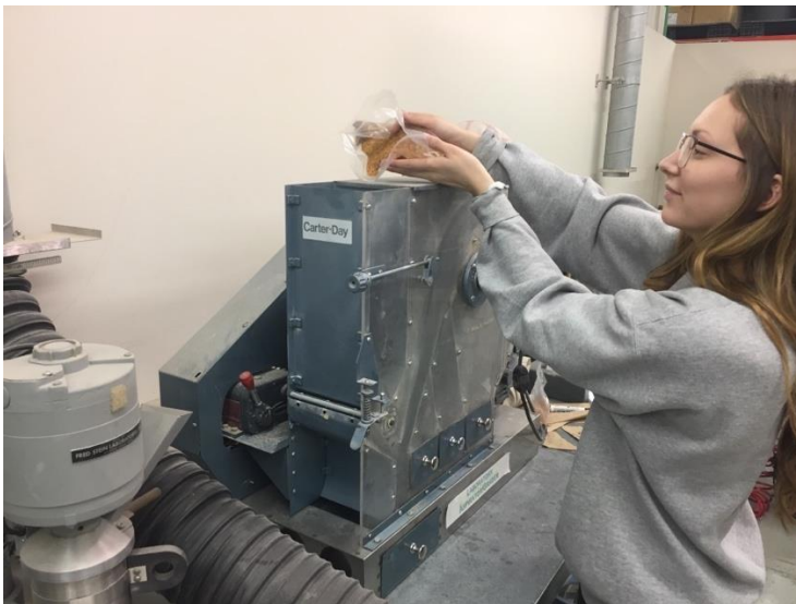
Figure 14. Small Carter Day laboratory air fractionator used for initial dehulling experiments.
