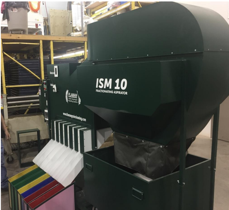
Figure 16. ISM 10 Fractionating aspirator used to produce bulk of hulls for steam treatment.
