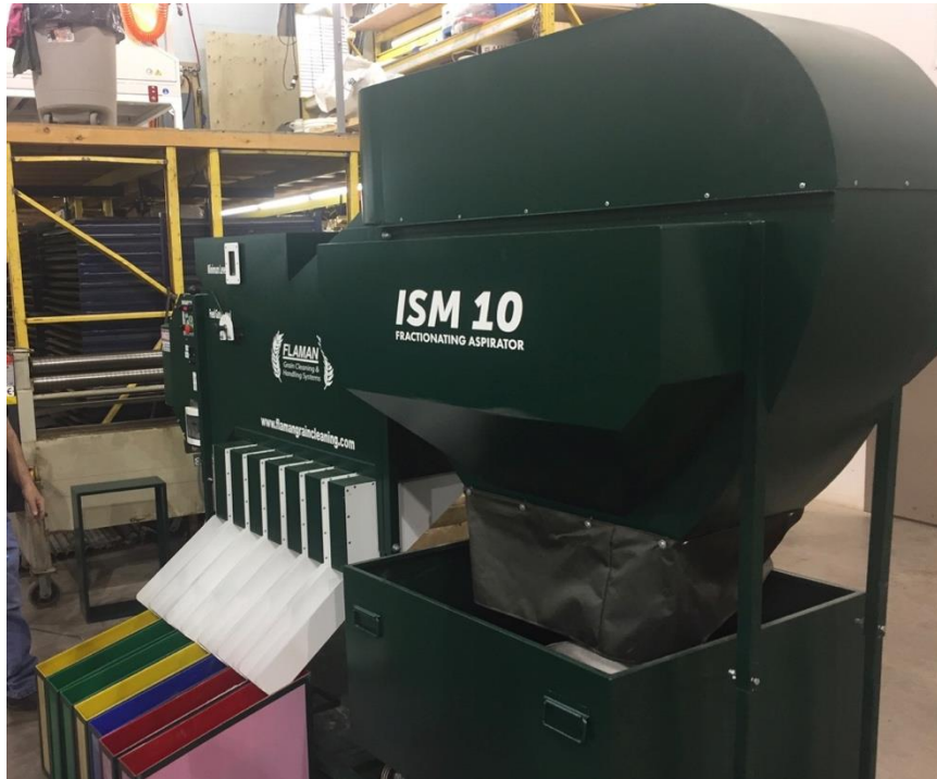
Figure 3.2 ISM 10 Fractionating aspirator used to separate the camelina hull from the cotyledon.
