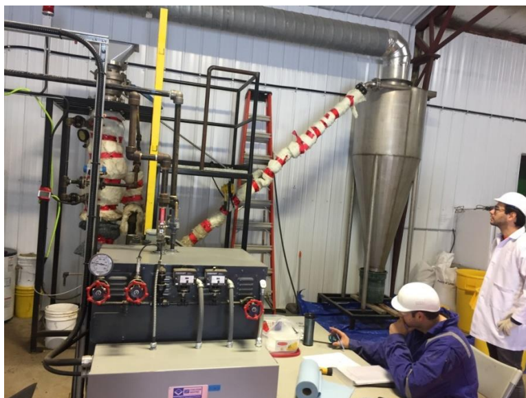
Figures 1& 2 Custom steam explosion system installed at the Canadian Feed Research Centre in North Battleford, SK
