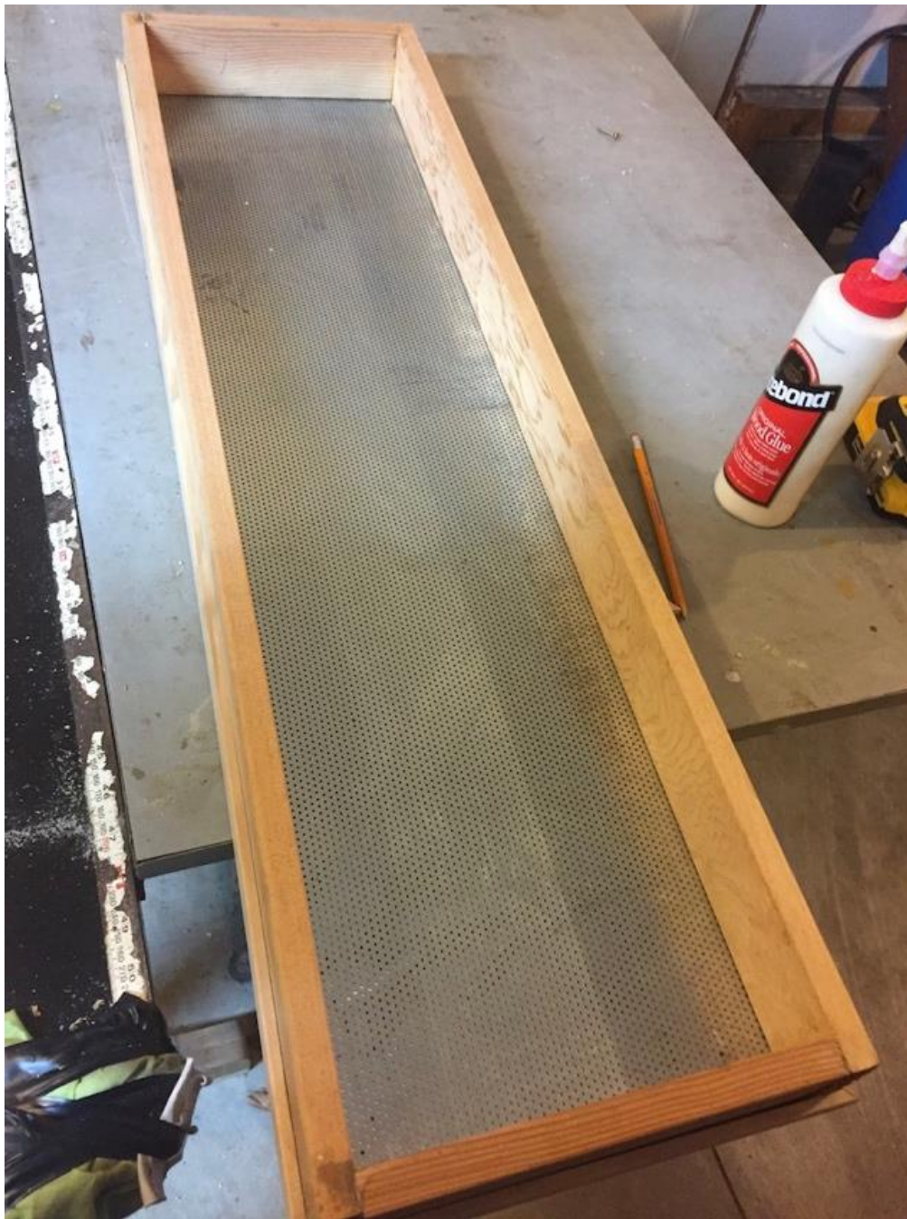
Figure 18. Custom sieve box used to separate hulls from cotyledons following air fractionation.
