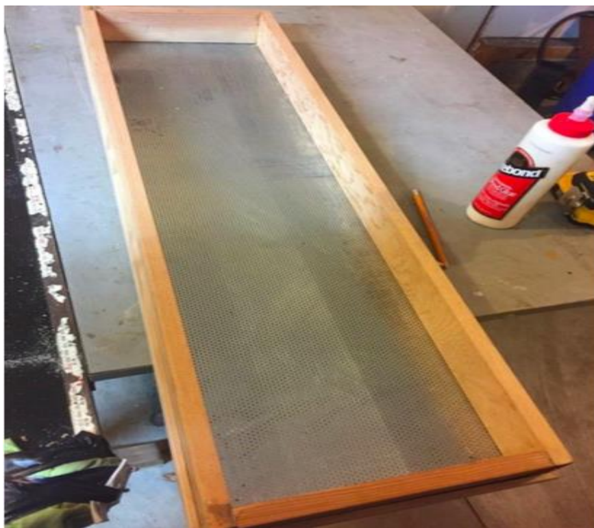
Figure 3.3 Custom sieve box used to purify the camelina hulls from cotyledons following air fractionation
