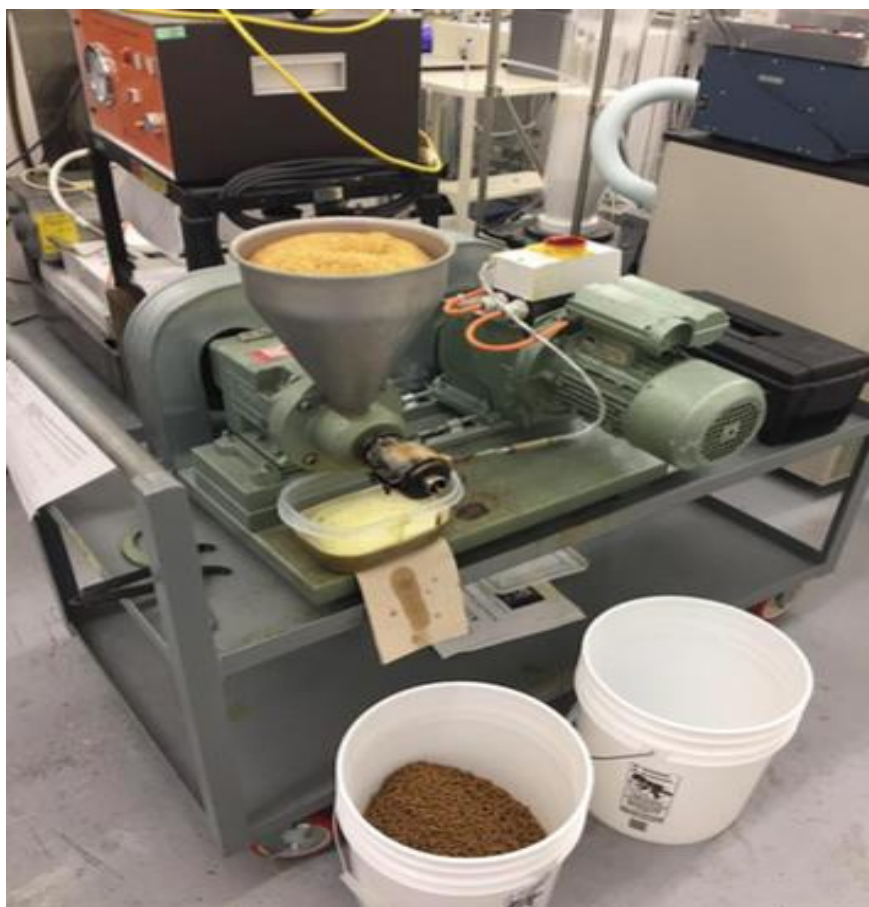
Figure 3 Expelling of dehulled camelina using a lab scale Komet oil expeller press
