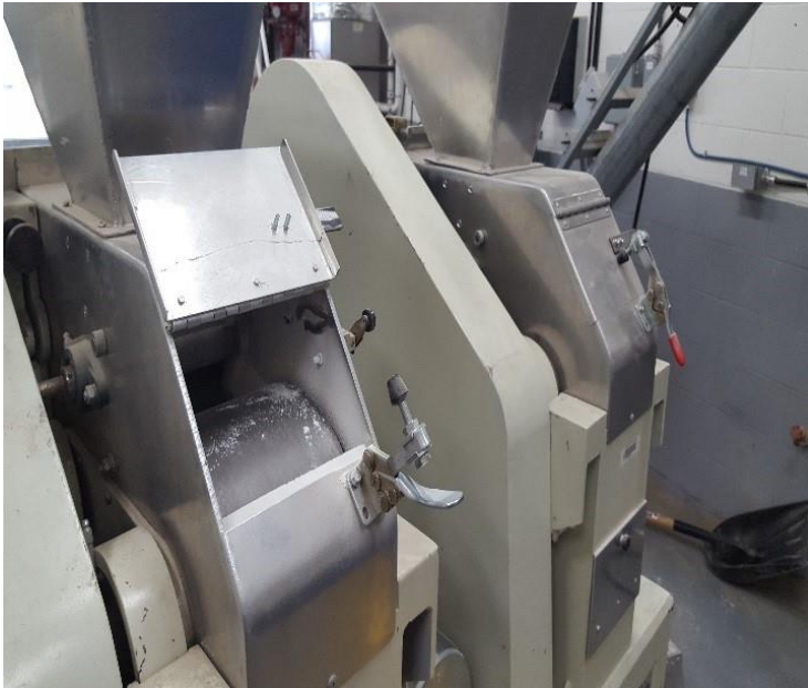
Figure 13. A custom roller mill equipped with smooth roles used to crack Canola, camelina and flax seeds during dehulling.
